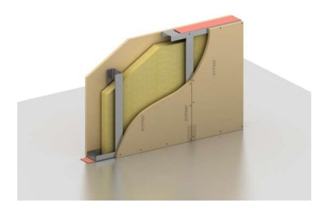
1 TP 11 AYSIST® Partition Wall System is built by screwing single layer of Aypan plasterboard to both sides of a metal single framework(DC) as indicated conditions in its technical specifications. The system contains insulation panels (rock wool divisionboard) inside selected in accordance with the length of the wall and the required insulation properties.
